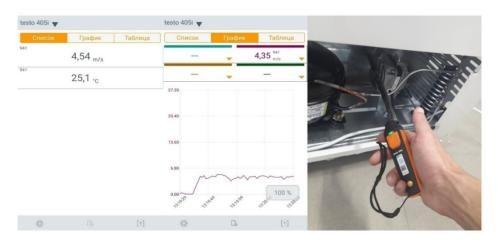
Figure 6 – Air speed measuring at the compressor compartment
