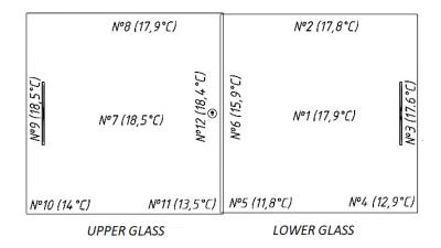
Figure 2 – The placement of thermometers and temperature indicators on glass doors
