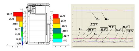
Figure 7 – Graphs of temperature dependence on time at the bottom of the pilot plant:  $W_{amb.}$  – related humidity;  $W_{given}$  – given related humidity;  $T_{amb.}$  – ambient temperature;  $T_{given}$  – given ambient temperature
