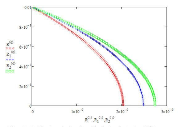
Figure 3 – And the change in the radius of the droplets for the three initial temperatures 493 K (220°C)  $2.031\cdot10^{-9}$  seconds 593 K (320°C)  $2.482\cdot10^{-9}$  seconds 693 K (420°C)  $2.741\cdot10^{-9}$  seconds
