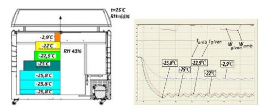
Figure 10 – Temperature reading and graph of temperature dependence on time in the refrigerated volume:  $W_{amb.}$  – related humidity;  $W_{given}$  – given related humidity;  $T_{amb.}$  – ambient temperature;  $T_{given}$  – given ambient temperature
