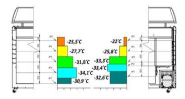
Figure 8 – Temperature reading from evaporator (leaf tube)
