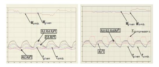
Figure 5 – Graph of temperature reading versus time in the shell of the low-temperature refrigerated case and in the compressor compartment:  $W_{amb.RH}$  – related humidity;  $W_{givenRH}$  – given related humidity;  $T_{amb.}$  – ambient temperature;  $T_{given}$  – given ambient temperature;  $T_{compressor\ com.}$  – temperature at te compressor compatiment.  $T_{compressor\ c.}$  =35.2°C
