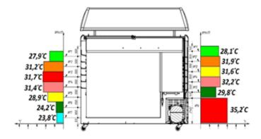
Figure 4 – Temperature reading in the shell of the refrigerated display case.
